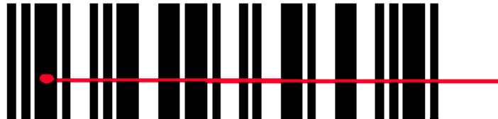
Figure 8-3 : Example of too small aperture size
